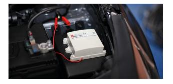
The **Human Detector** Sensor is hidden in the automobile. No complicated installation is required, as is the case with other alarm systems. The sensors comprise a battery, and transmit information via radio. Each installation is capable of monitoring up to 1000 vehicles.
